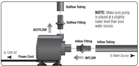
**EXAMPLE 4: Inline Application with Garden Hose Adapter** (Select Models Only) Secured pump NOT submerged in water and operating without the Strainer, Filter and Cover installed.
