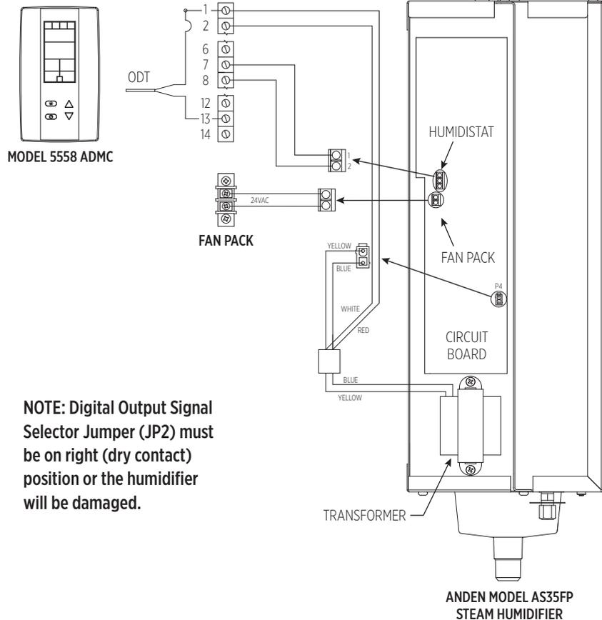
**NOTE:** Digital Output Signal Selector Jumper (JP2) must be on right (dry contact) position or the humidifier will be damaged.
