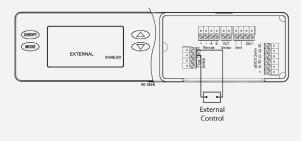
The Model A710 can be controlled with the Model A77 Control (included) or any external control that can provide a dry contact closure. When the Model A77 is used, the User Interface on the dehumidifier **MUST BE** set to "Remote". For all other external controls, the User Interface **MUST BE** set to "External". Refer to the quick start guide or installation manual for instructions on accessing the installer set-up menu.
