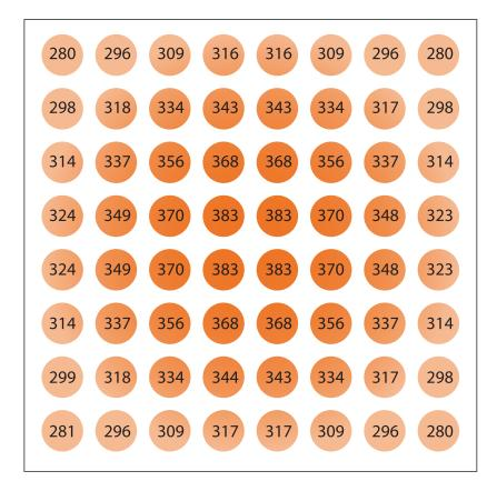
**Note:** Photosynthetic Photon Flux Density (PPFD) data is produced by using professional lighting simulation software and third party laboratory photometric files. All PPFD data are measured in µmol/m²/s. The result assumes a single fixture being mounted in a 4'x4' grow tent with 85% wall reflectance. Actual measurement may vary depending on actual use conditions, input voltages, and measuring instruments. Professional lighting plans for commercial applications are available upon request.
