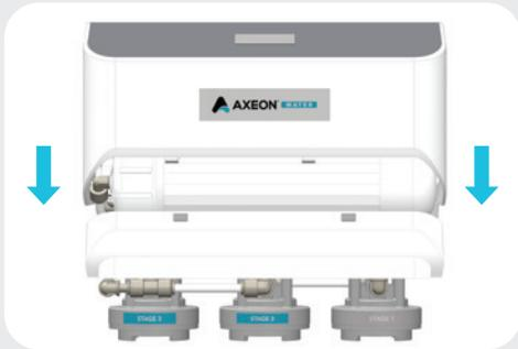
**Step 1H:** Re-install the cover. Engage the tabs located in the back. Make sure the power cables connected to the cover are aligned in the middle of the cover and that the membrane housings are aligned to allow the cover to sit properly. Next, re-install the screws that secure the cover.
