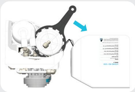
**Step 1G:** Re-install the end cap by turning it in a clockwise direction until firmly tightened. Reconnect the tubing to the cap and re-install the locking cotter clips. Be careful that you do not over-tighten, pinch, or cut any O-rings when re-installing the end caps.
