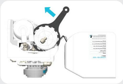
**Step 1D:** Disconnect the locking cotter clips and tubing going to the HyperFilter housing cap, then unscrew the cap, using the included wrench, in a counterclockwise direction. Repeat this step for the 2<sup>nd</sup> HyperFilter housing.
