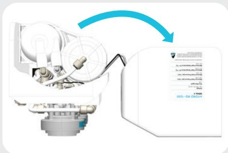
**Step 1C:** GENTLY lift the cover upwards only a few inches, then carefully lean the top towards yourself, flipping it upside down so it lays on its topside.
