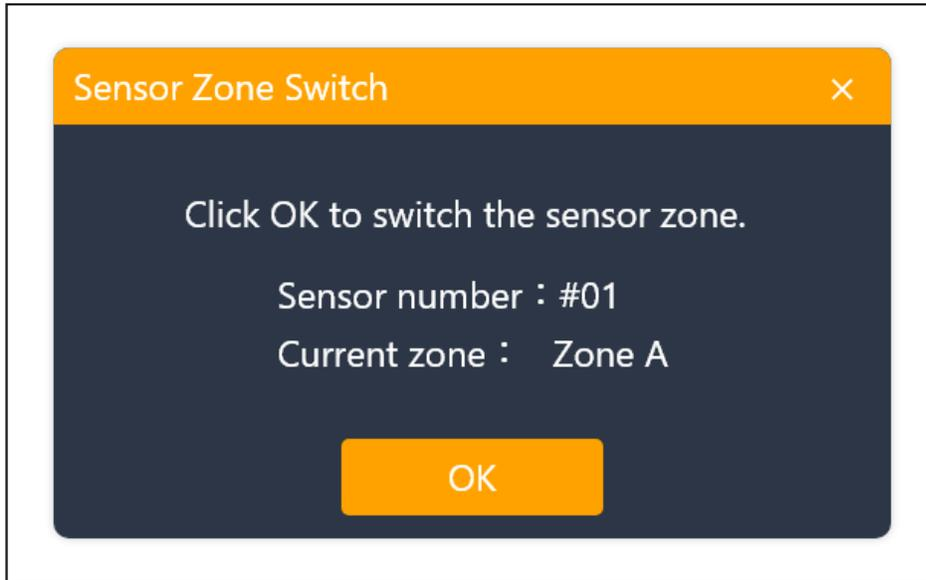
Sensor Locating: Click "OK," and the indicator on the sensor will start flashing. Use it to confirm the physical location of the sensor.
