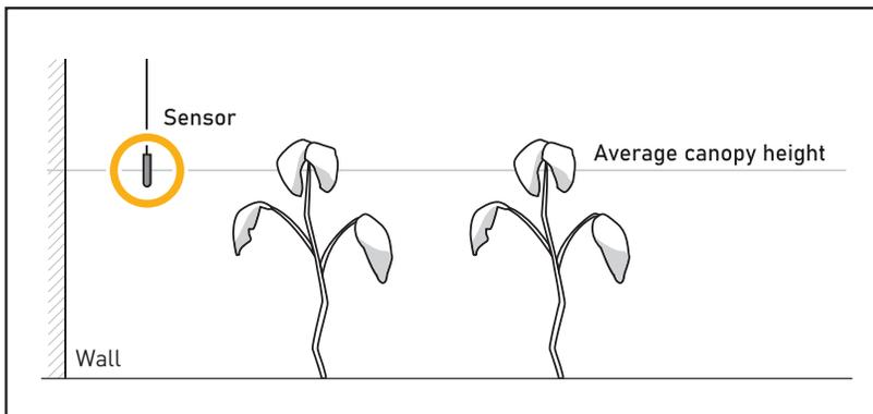
If there is a sensor for your HVAC system, install the controller near the sensor for that system. If necessary, the sensor cable can be extended by 5 meters using a standard 3.5 mm jack extension cable. Sensors with a cable length of 30 meters are also available (HGC906196).
