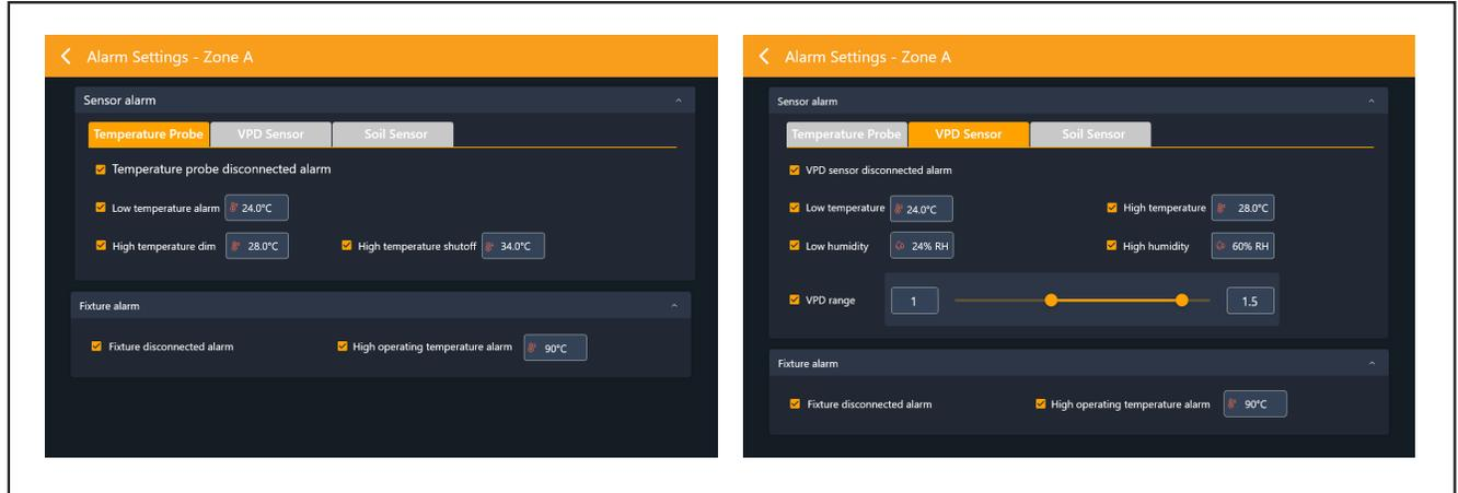
Low temperature alarm: When the room temperature is lower than the value set by the user, a warning with an alert box and an alarm message will be added to the alarm log page.
