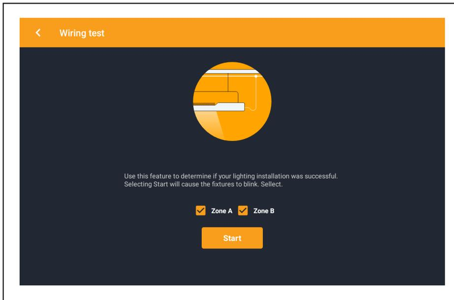
Click "Start" to begin the test. After the test starts, all the lights on the line will switch between on and off for five seconds. The user can judge whether the lights are normal or not according to the fixture behavior:
